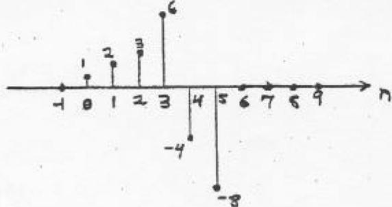
For this problem, aliasing means the last three points ( $n = 4, 5, 6$ ) will wrap-around on top of the first three points, giving  $y[n] = x[n] * h[n]$ :
