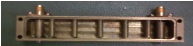
Figure 8. A five poles comblin filter
