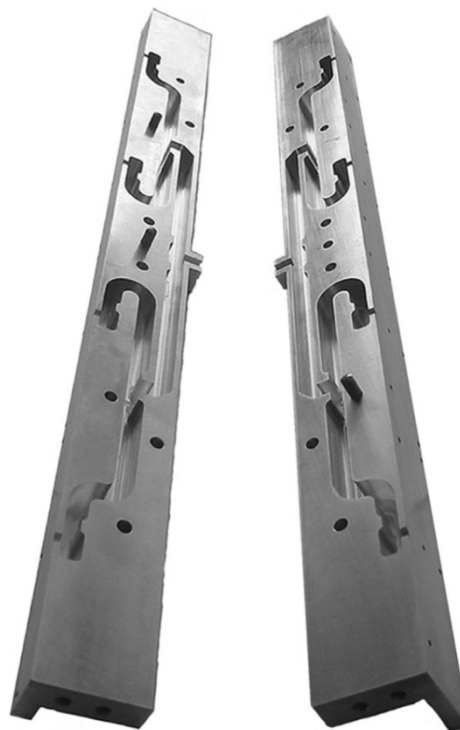
Fig. 11. CNC-milled two-piece waveguide feed system.
