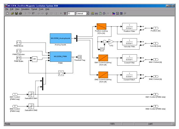
Fig. 28. Interior of the driver block
