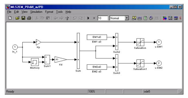
Fig. 45. Interior of the PD differential controller
