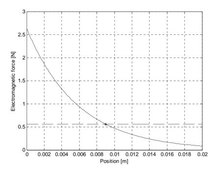
Fig. 38. Electromagnetic force vs. position. The gravity force of the big ball (dashed horizontal line) is crossing the curve at the 0.009 m distance from the electromagnet
