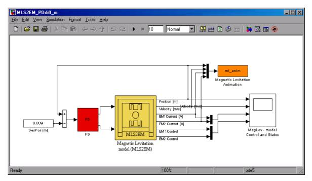
Fig. 44. PD differential mode simulation
