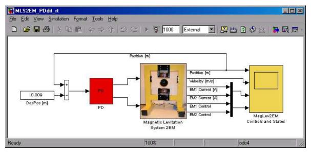
Fig. 52. PD differential control real-time experiment.
