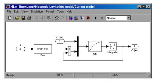
Fig. 35. Interior of the Current model block
