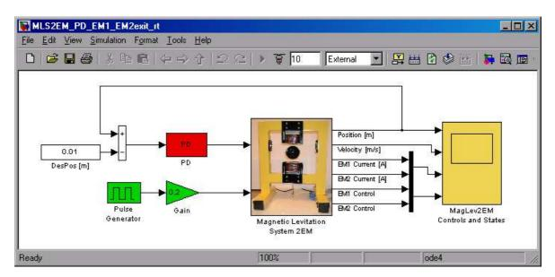
Fig. 50. PD control and pulse excitation real-time experiment.
