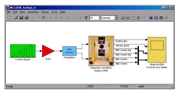
Fig. 24. Real-time model built to examine EMF influence on the coil current
