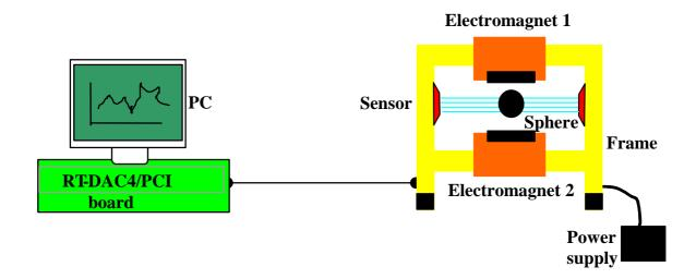
Fig. 1. MLS2EM laboratory set-up
