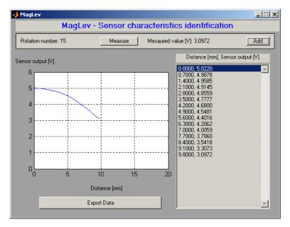
Fig. 5. Characteristics of the sphere position sensor
