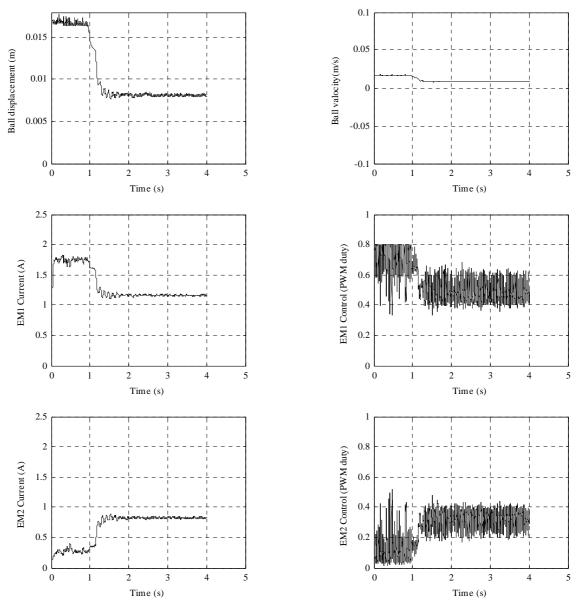
Fig. 53. PD operating in differential mode real-time experiment. The desired position as a constant.
