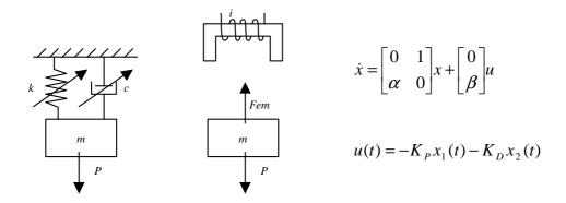
The closed loop system has two poles which can be located on the imaginary axis representing the marginally stable system but generally they are located in the left half plane to obtain desired performance. Choosing appropriate values of poles we can obtain the required dynamic behavior of the closed loop system.
