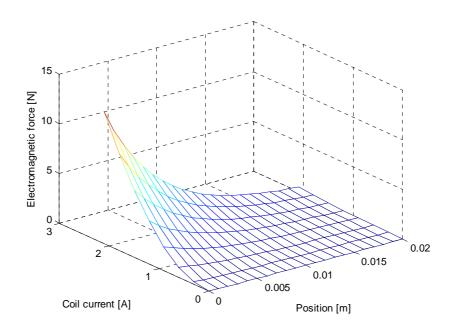
Fig. 40. Electromagnetic force vs. coil current and distance from the electromagnet.
