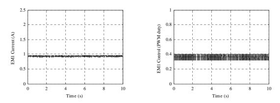
Fig. 43. PID simulation – the desired position is a constant.
