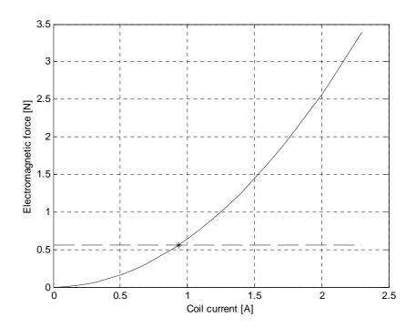
Fig. 39. Electromagnetic force vs. coil current. The gravity force of the big ball (dashed horizontal line) is crossing the curve at the 0.9345 A coil current
