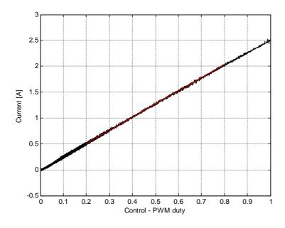
Fig. 17. Current vs. PWM duty cycle
