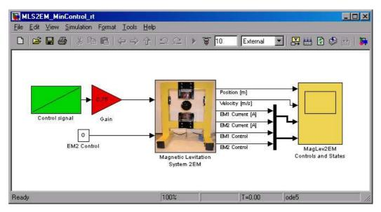
Fig. 19. Real-time model built to examine the minimal electromagnetic force
