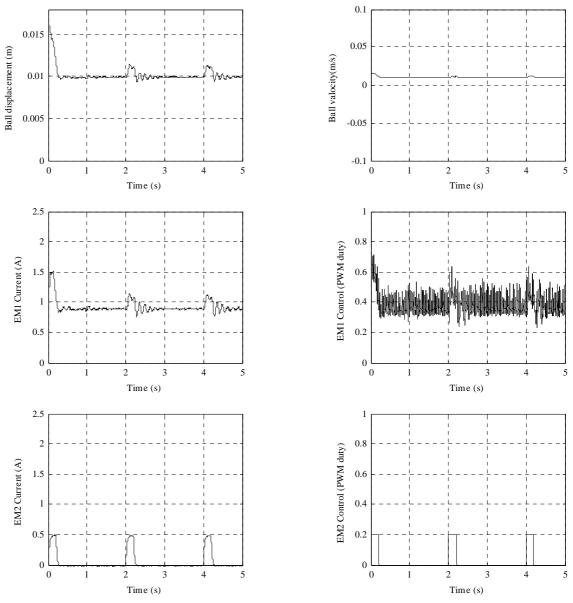
Fig. 51. PD stabilization and external pulse type excitation real-time experiment. The desired position as a constant.
