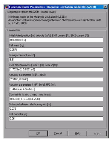
Fig. 33. Mask of the Magnetic Levitation model MLS2EM
