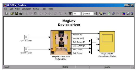
Fig. 27. RTWT MagLev device driver window
