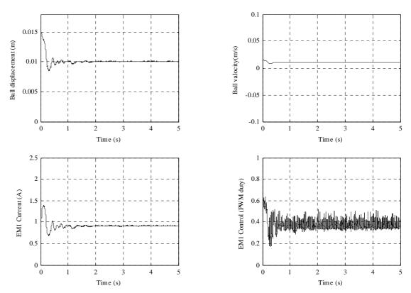
Fig. 49. PD real-time experiment. The desired position as a constant.
