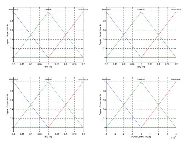
Fig. 6.13 Membership function for  $dH_1$ ,  $dH_2$ ,  $dH_3$  and pump control signals
