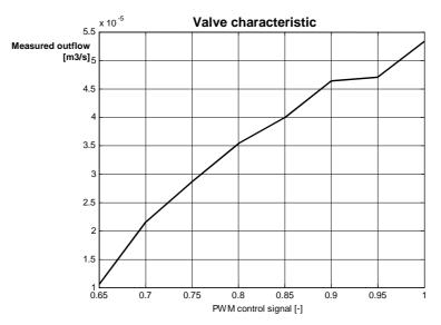
Fig. 5.2 Controlled valve characteristic
