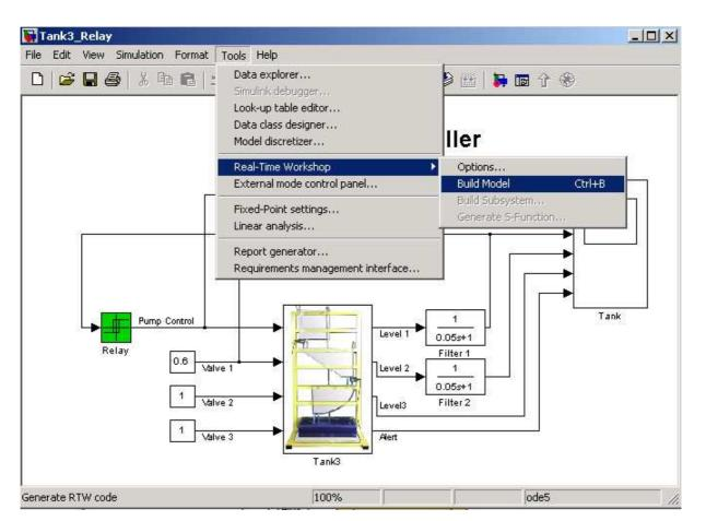
Fig. 7.1 Creating the executable file under RTWT
