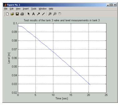
Fig. 2.7 Level in tank 3 (valve 3 is opened)
