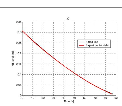
Fig. 5.6 The upper tank identification: C1 = 5.6578e-005, Alfa1 = 0.2900
