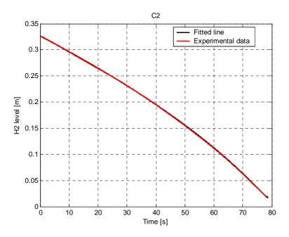
Fig. 5.7 The middle tank identification: C2 = 5.5800e-005, Alfa2 = 0.2256
