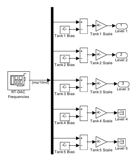
Fig. 3.6 The level sensor characteristic curve built into the device driver (Tank4 and Tank5 are not used)
