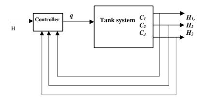
Fig. 4.5 Pump controlled system, closed loop
