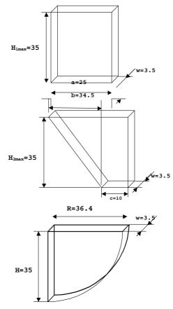
Fig. 4.4 Geometrical parameters of the tanks
