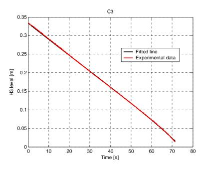
Fig. 5.8 The lower tank identification: C3 = 7.4102e-005, Alfa3 = 0.2487
