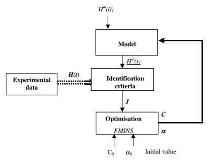
Fig. 5.5 Principle of tank parameters identification
