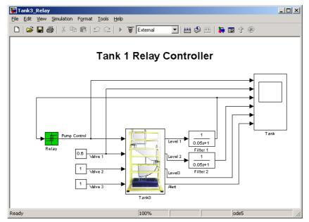
Fig. 3.7 Control system with relay controllers
