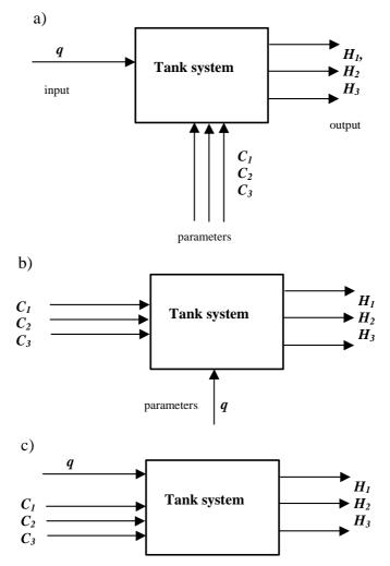
Fig. 4.2 Models of the tank system as: a) pump-controlled system, b) valve-controlled system c)pump/valve controlled system.
