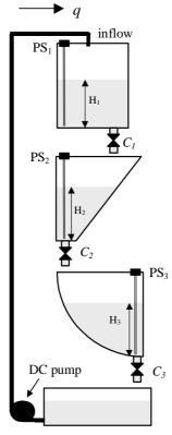
Fig. 4.1 Configuration of the multitank system
