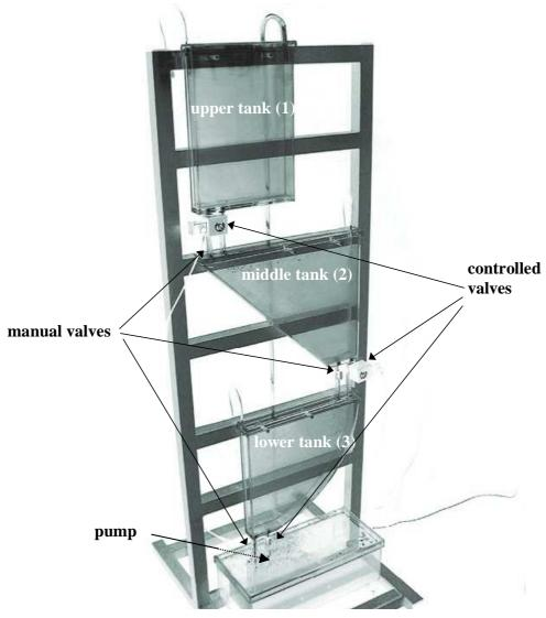
Fig. 1.1 Multitank system
