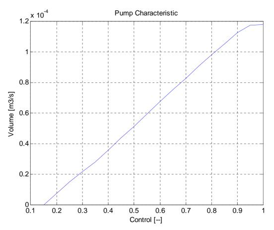
Fig. 5.4 DC pump characteristic curves measured for PWM frequency 300 Hz (*PWMPrescaler=31* and *12-bit mode*)
