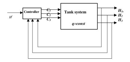
Fig. 4.6 Valve-controlled system, closed loop
