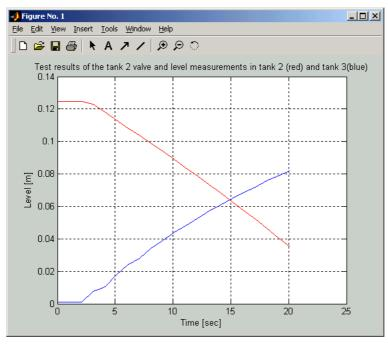
Fig. 2.6 Levels in the tank2 and 3 (valve 2 is opened)
