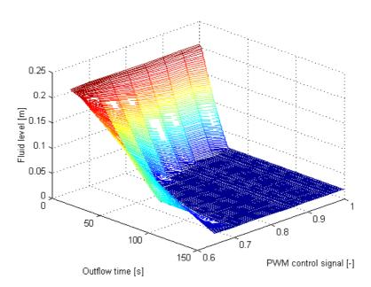
Fig. 5.3 Time characteristic curve of the valve
