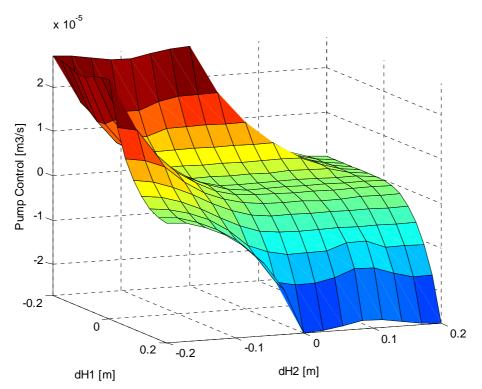
Fig. 6.12 Pump control surface versus  $dH_1$  and  $dH_2$  input signals
