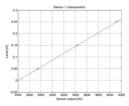
Fig. 5.1 Pressure sensor characteristic. Red points-measurements, solid line-fitting line
