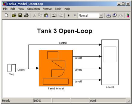
Fig. 3.2 The triple tanks system simulation model
