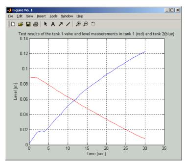
Fig. 2.5 Levels in the tanks 1 and 2 (valve 1 is opened)
