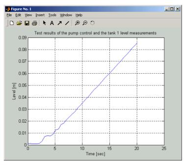
Fig. 2.4 The proper operation of the sensors: level in the tank 1 (the pump works and valve 1 is closed)
