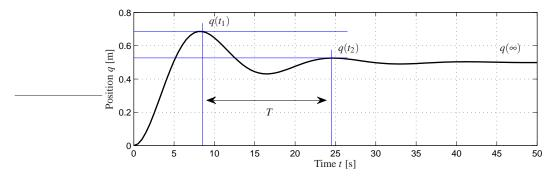
**Figure 2.14:** Step response for a spring-mass system. The magnitude of the step input is  $F_0 = 20$  N. The period of oscillation, T is determined by looking at the time between two subsequent local maxima in the response. The period combined with the steady state value  $q(\infty)$  and the relative decrease between local maxima can be used to estimate the parameters in a model of the system.
