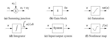
**Figure 2.12:** Standard block diagram elements. The arrows indicate the inputs and outputs of each element, with the mathematical operation corresponding to the blocked labeled at the output. The system block (e) represents the full input/output response of a dynamical system.
