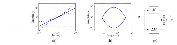
**Figure 2.15:** Characterization of model uncertainty. Uncertainty of a static system is illustrated in (a). The uncertainty lemon in (b) is one way to capture uncertainty in dynamical systems emphasizing that a model is only valid in some amplitude and frequency ranges. In (c) a model is represented by a nominal model (M) and another model  $\Delta M$  representing the uncertainty analogous to representation of parameter uncertainty.
