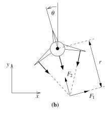
**Figure 2.17:** Vectored thrust aircraft. The Harrier AV-8B military aircraft (a) redirects its engine thrust downward so that it can "hover" above the ground. Some air from the engine is diverted to the wing tips to be used for maneuvering. As shown in (b), the net thrust on the aircraft can be decomposed into a horizontal force  $F_1$  and a vertical force  $F_2$  acting at a distance r from the center of mass.
