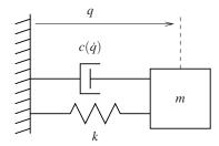
**Figure 2.1:** Spring-mass system, with nonlinear damping. The position of the mass is denoted by q, with q = 0 corresponding to the rest position of the spring. The forces on the mass are generated by a linear spring with spring constant k and a damper with force dependent on the velocity  $\dot{q}$ .
