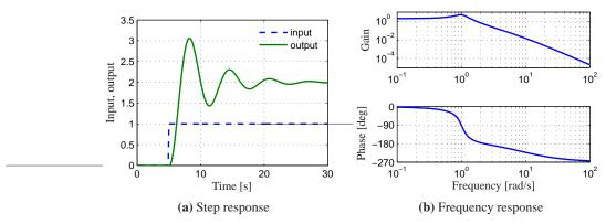
**Figure 2.4:** Input/output response of a linear system. The step response (a) shows the output of the system due to an input that changes from 0 to 1 at time t = 5 s. The frequency response (b) shows the amplitude gain and phase change due to a sinusoidal input at different frequencies.
