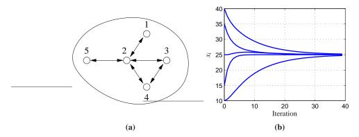
**Figure 2.21:** Consensus protocols for sensor networks. A simple sensor network with five nodes is shown on the left. In this network, node 1 communicates with node 2, node 2 communicates with notes 1, 3, 4 and 5, etc. A simulation demonstrating the convergence of the consensus protocol (2.31) to the average value of the initial conditions is shown on the right.
