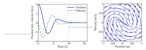
**Figure 2.2:** Illustration of a state model. A state model gives the rate of change of the state as a function of the state. The plot on the left shows the evolution of the state as a function of time. The plot on the right shows the evolution of the states relative to each other, with the velocity of the state denoted by arrows.
