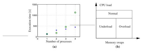
**Figure 2.20:** Illustration of feedback in the virtual memory system of IBM/370. The left figure (a) shows the effect of feedback on execution times in a simulation, following [BG68]. Results with no feedback are shown with 0 and with feedback with x. Notice the dramatic decrease in execution time for the system with feedback. The right figure (b) illustrates how the three states were obtained based on process measurements.
