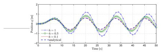
**Figure 2.9:** Simulation of the forced spring-mass system with different simulation time constants. The darker dashed line represents that analytical solution. The solid lines represent the approximate solution via the method of Euler integration, using decreasing step sizes.
