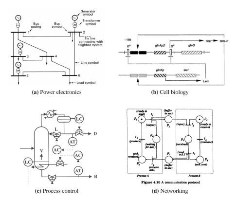
**Figure 2.11:** Schematic diagrams in different disciplines. Each diagram is used to illustrate the dynamics of a feedback system: (a) electrical schematics for a power system, (b) a biological circuit diagram for a synthetic clock circuit [ASMN03], (c) process diagram for a distillation column and (d) Petri net description of a communication protocol [?].
