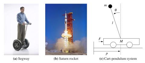
**Figure 2.5:** Balance systems. (a) Segway human transportation system, (b) Saturn rocket and (c) inverted pendulum on a cart. Each of these examples uses forces at the bottom of the system to keep it upright.
