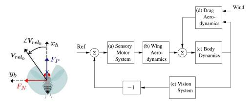
**Figure 2.13:** A block diagram representation of the flight control system for an insect flying against the wind. The mechanical portion of the model consists of the rigid body dynamics of the fly, the drag due to flying through the air and the forces generated by the wings. The motion of the body causes the visual environment of the fly to change, and this information is then used to control the motion of the wings (through the sensory motor system), closing the loop.
