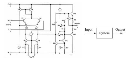
**Figure 2.3:** Illustration of the input/output view of a dynamical system. The figure on the left shows a detailed circuit diagram for an electronic amplifier; the one of the right its representation as a block diagram.
