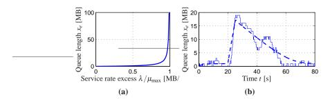
**Figure 2.19:** Queuing dynamics. The figure on the left shows steady state queue length as a function of  $\lambda/\mu_{\text{max}}$ , and the figure on the right shows the behavior of the queue length when there is a temporary overload in the system. The full line shows a realization of an event based simulation and the dashed line shows the behavior of the flow model (2.29).
