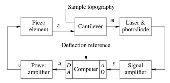
**Figure 3.15:** Block diagram of the system for vertical positioning of the cantilever for an atomic force microscope (AFM) in scanning mode. The control system attempts to keep the cantilever deflection equal to it reference value. Cantilever deflection is measured, amplified and converted to a digital signal, then compared with its reference value. A correcting signal is generated by the computer, converted to analog form, amplified and sent to the piezo element.
