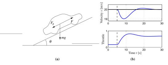
**Figure 3.3:** Car with cruise control encountering a sloping road: a schematic diagram is shown in (a) and (b) shows the response in speed and throttle when a slope of  $4^{\circ}$  is encountered. The hill is modeled as a net change in hill angle,  $\theta$ , of 4 degrees, with a linear change in the angle between t = 5 and t = 6. The PI controller has proportional gain is  $k_p = 0.5$  and the integral gain is  $k_i = 0.1$ .
