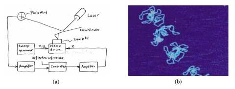
**Figure 3.14:** Atomic force microscope. A schematic diagram of an atomic force microscope is shown on the left, consisting of a piezo drive that scans the sample under the AFM tip. A laser reflects off of the cantilever and is used to measure the detection of the tip through a feedback controller. An AFM image of DNA is shown on the right.
