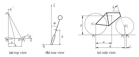
**Figure 3.5:** Schematic views of a bicycle. The steering angle is  $\delta$ , the roll angle is  $\varphi$ . The center of mass has height *h* and distance *a* from a vertical through the contact point *P*<sub>1</sub> of the rear wheel. The wheel base is *b* and the trail is *c*.
