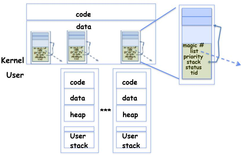
Each user process/thread associated with a kernel thread, described by a 4kb Page object containing TCB and kernel stack for the kernel thread
