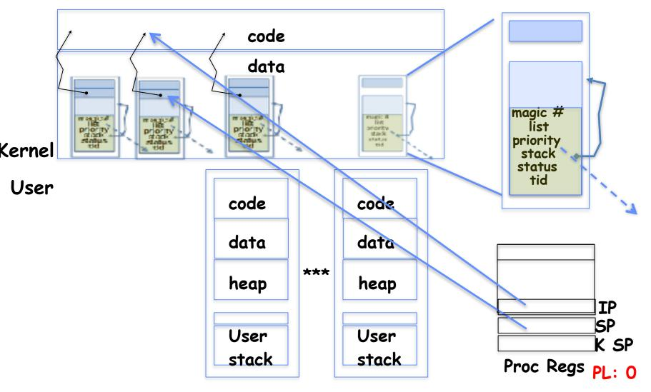
switch\_threads: save regs on current small stack, change SP, return from destination threads call to switch\_threads
