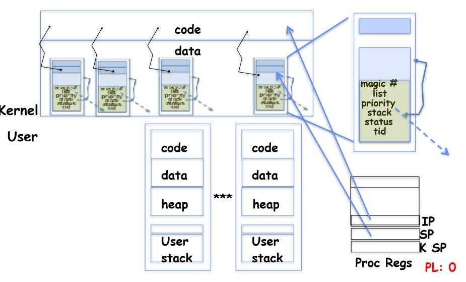
• Mechanism to resume k-thread goes through interrupt vector
