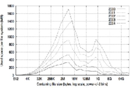
Fig. 4. Histograms of bytes by containing file size.
